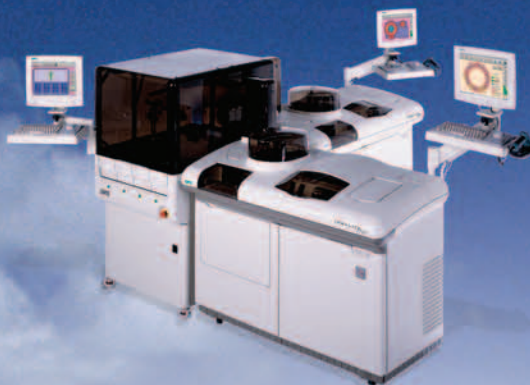
Figure 2. An example of an island of automation is the DPC Immunoassay Workcell. Here the Sample Management System (SMS) connects two IMMULITE 2500 systems, providing the lab with a single sample-entry point and access to 48 different analytes.
